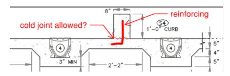
Answer: The construction method shown above will be allowed, and any costs should be included in Bid Item 7 - Concrete Slab. Reinforcement size and spacing is to be approved by the Project Manager.
