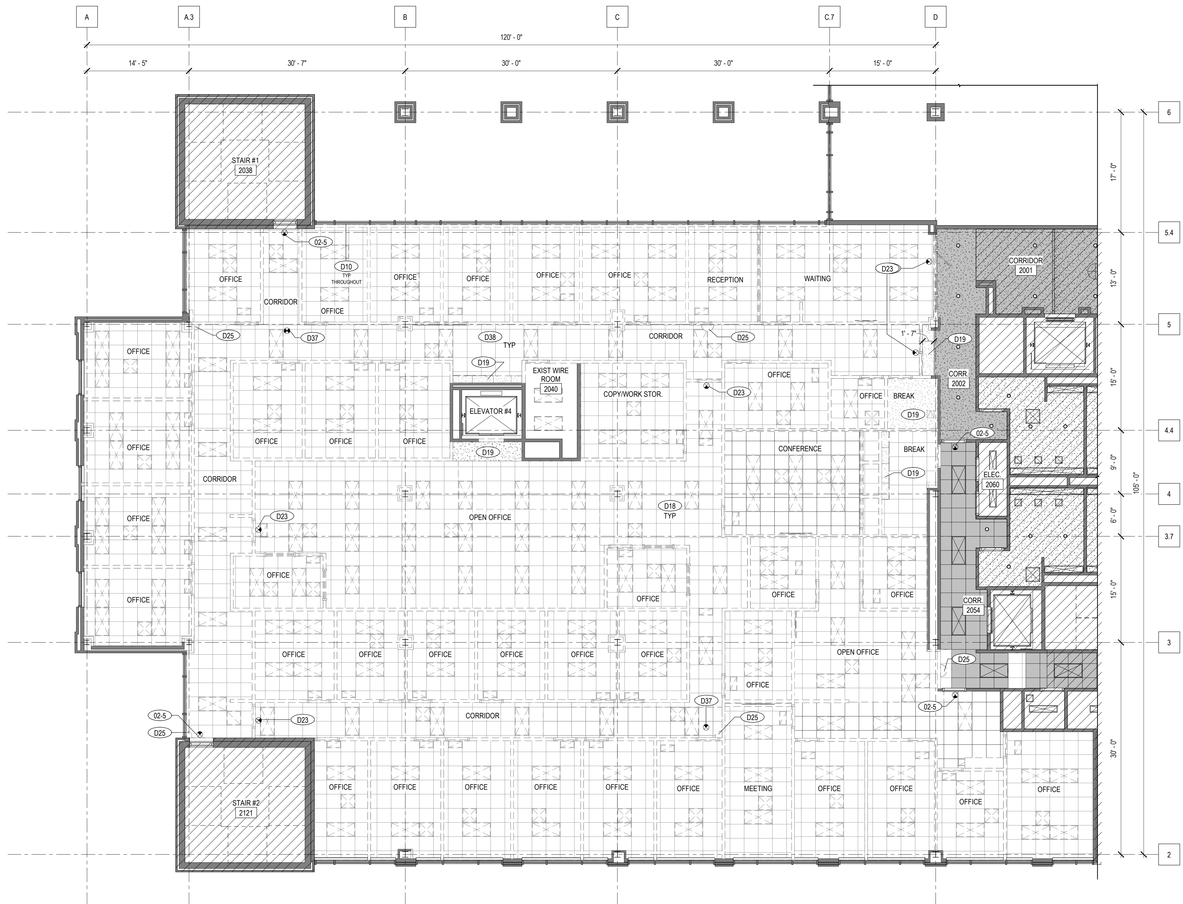
DEMOLITION REFLECTED CEILING PLAN AD6-1 1/8" = 1'-0" NORTH
